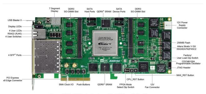
\*Cypress QDRII+ SRAM or functional compatible SRAMS provided by GSI (SigmaQuad-II+) and ISSI (QUADP).
